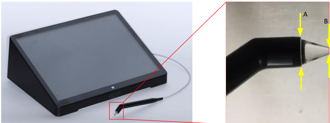
Figure 2.9 The clinical system prototype hardware implementation, (left) the unit, (right) the probe tip - conical delay line with A = 12 mm and B = 1.5 mm.
