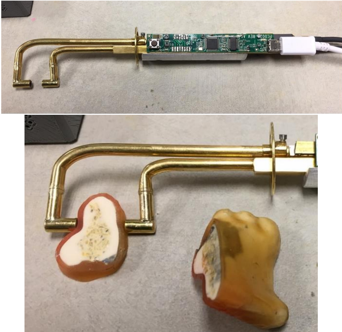
Figure 6.5 The third prototype equipped with a custom, developed an electronic board for proximity data acquisition highlighted in Figure 6.2.
