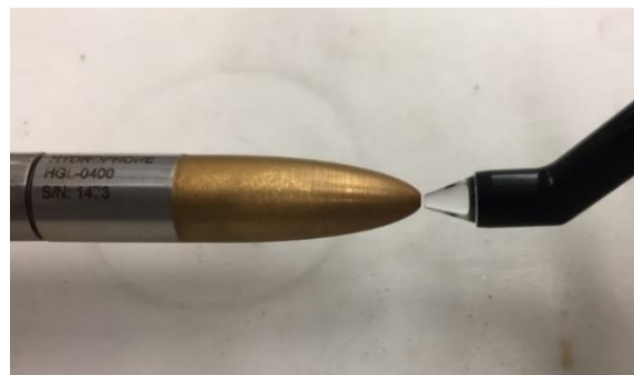
Figure 7.4 The hydrophone and the evaluated probe lined up in the testing tank.
