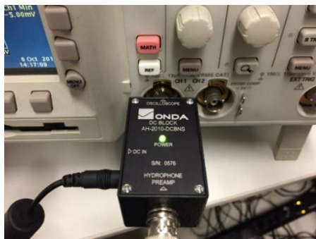
Figure 7.3 Pre-amplifier connected directly to the oscilloscope.
