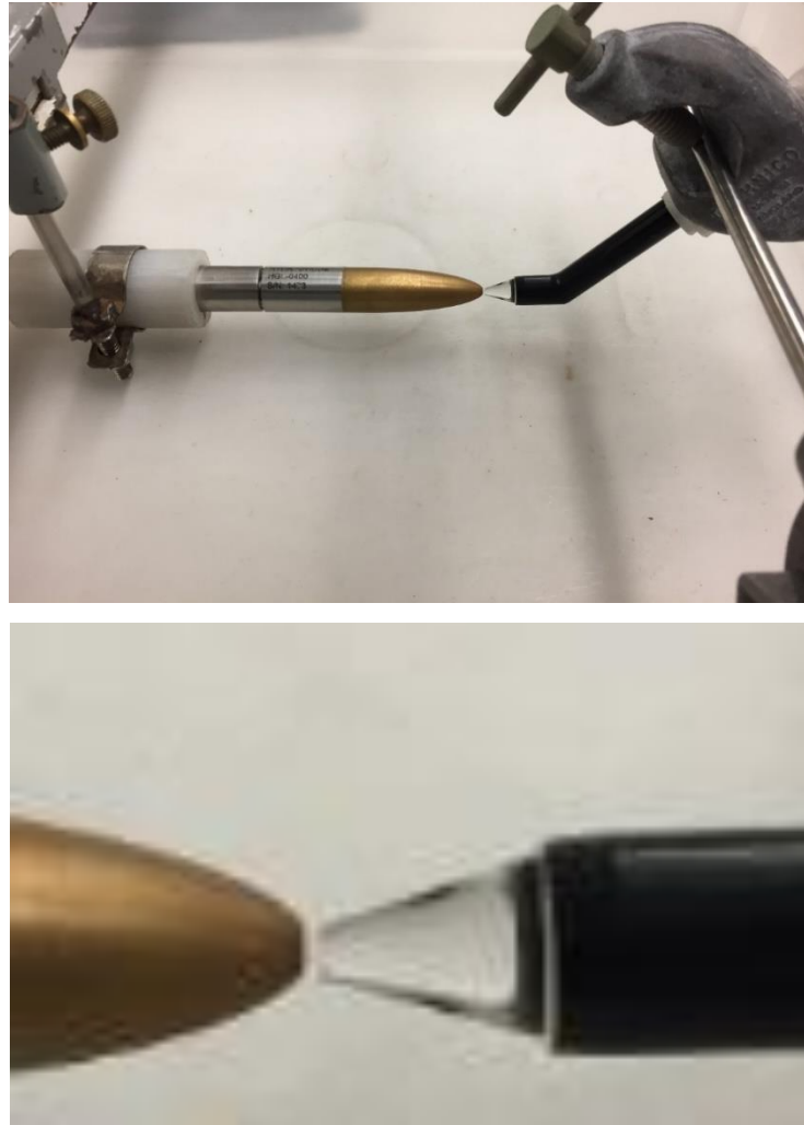
Figure 7.2 Acoustic output measurement setup.
